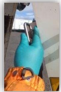
Simulation of Operative's hand that was caught between the locking pin and boom
