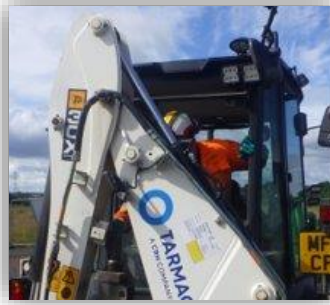
Simulation of Operative attempting to install the locking pin from the cab
