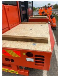
Following consultation with the hirer, timber bearers were securely fitted to the deck of the FLT using the manufacturers pre-drilled holes.
