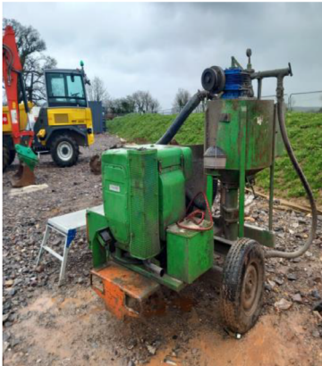
The Colmono CX410 Colloidal grout plant on site
