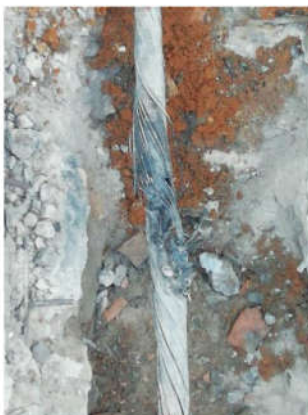
Picture 3 – Visible indication of the struck cable when the temporary door is open
