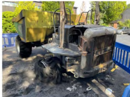
Dumper following fire
