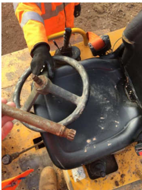
Damaged Steering wheel and column
