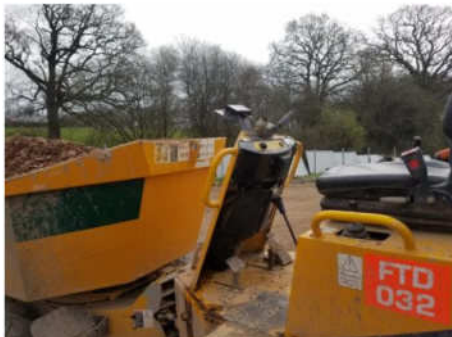
Damaged and missing steering column on 3T dumper
