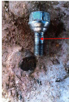
Wheel stud with 50% of thread damaged
