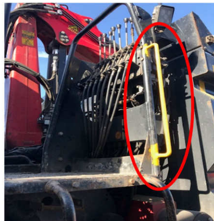
The highlighted area shows the new handrail for better access
