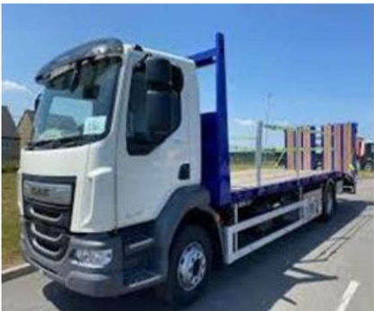
Figure 2: Beaver Tail style Lorry used to move excavator
