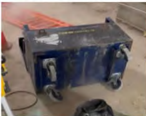
Picture 4 – Box that fell next to a similar size box – note the reduced width between the castors causing the instability of the box.
