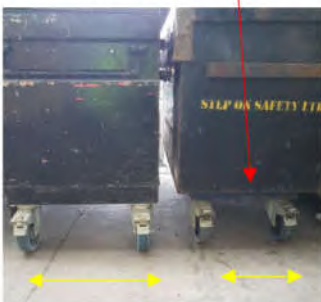
Picture 4 – Box that fell next to a similar size box – note the reduced width between the castors causing the instability of the box.
