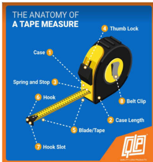
Pictures denote parts of a tape measure & the tape measure being used at the time of the accident.
