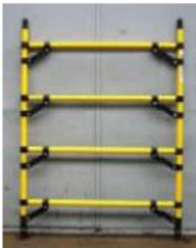
Modified 1450 span frame with additional gusset supports to each rung
