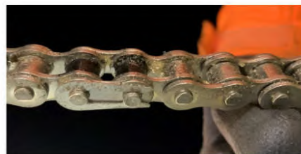
Photo: Correctly installed spring-clip on split-link
