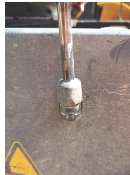
Image showing ram without retaining clip.
