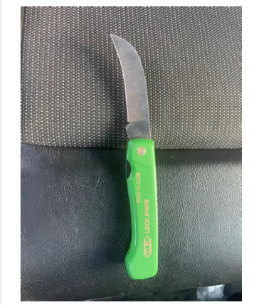
Folding blade knife used to cut ducting
