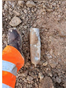
Approximate size of gas canister consistent with those used for Mig welding
