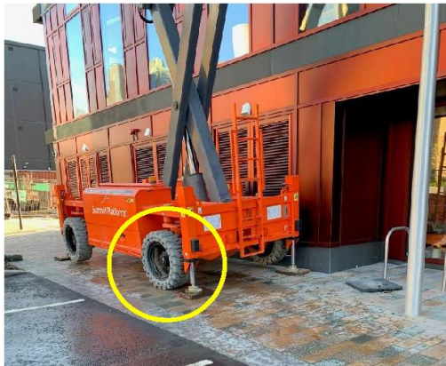
Jack leg shown has retracted causing the machine to rest on the wheel whilst extended to 20m height.
