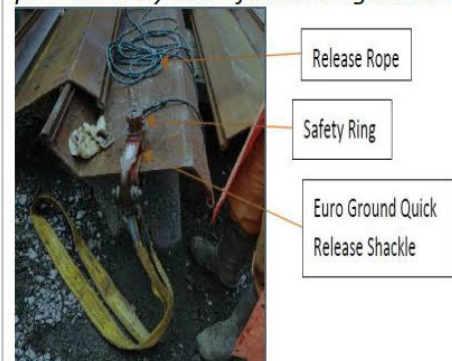
Fig. 2: Showing how the Shackle should have been installed correctly, as prescribed by manufacturer's guidance
