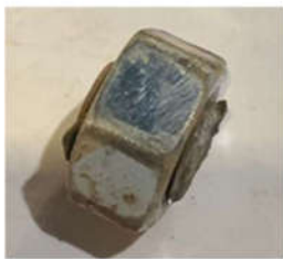
Formwork stud which failed within the thread.
