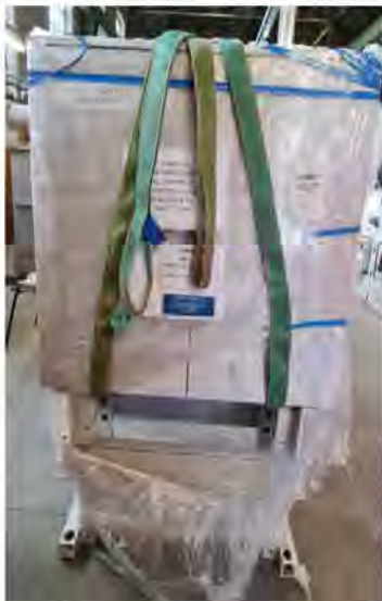
Image showing how the LCP was slung during the lifting operation
