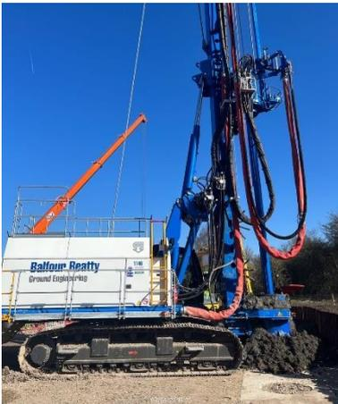
On Thursday 6 July 2023 at our AWE Aldermaston site, following the successful completion of concrete pumping on a Casagrande B300 continuous flight auger piling rig, the piling team commenced work to clean the concrete pumping system using compressed air. During this cleaning operation, a blockage was encountered.
